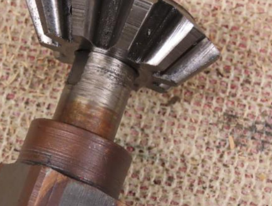
Seized shaft and planet gear showing galling on shaft
