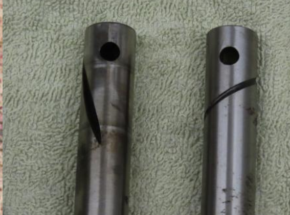
Late design of pinion shaft (left) and Club re-design (right)
