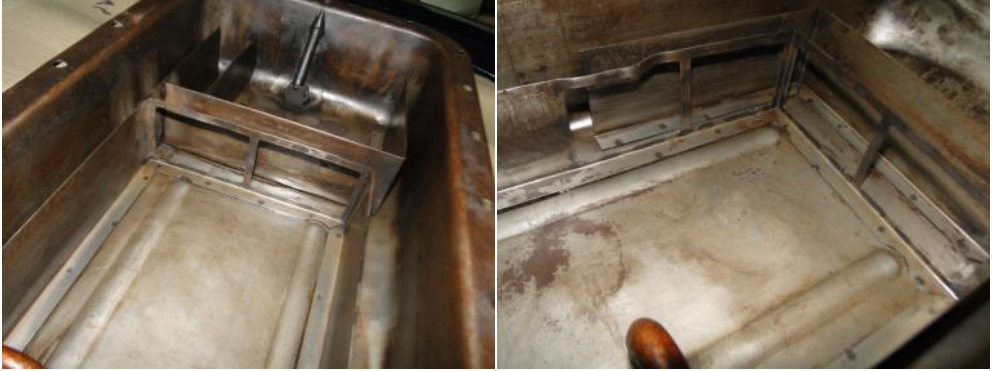
Mesh support baffles rear (left image) and front (right image) after removal of old mesh.
