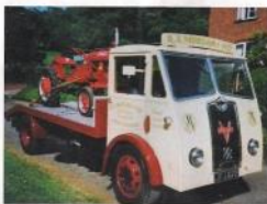
4 1949 Vulcan 6 PF lorry. Six cylinder Perkins engine. Four speed gearbox two speed axle. Beaver tail body and ramps. Purchased by John Onions of Shrewsbury then restored and overhauled by John Boughey. A rare lorry suit any collection. Reg no JFJ 672
