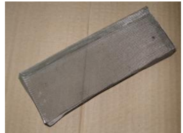
Mesh support baffles rear (left image) and front (right image) after removal of old mesh.
