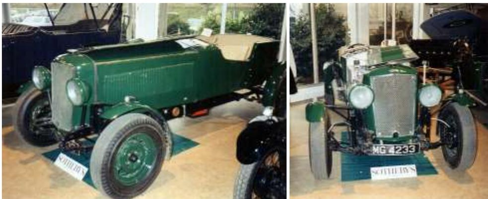
The reason the car now has a painted radiator surround is because it was being transported on a trailer without being strapped down(!) and car and trailer went separate ways, the former coming to a halt against a tree. The radiator surround could not be repaired sufficiently well to be chrome plated again, so there will likely be some filler underneath the paint. No Railton was ever supplied new with a painted radiator surround.
